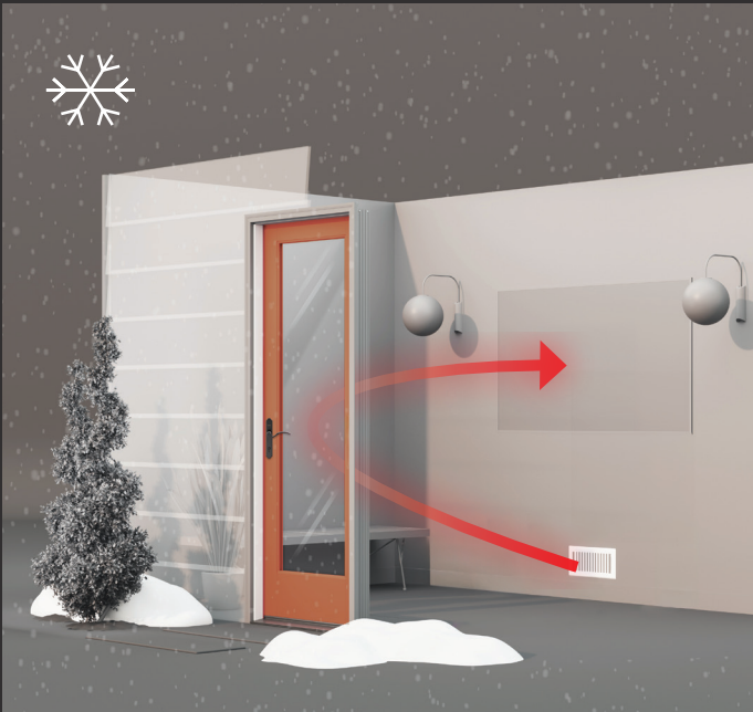
In cold weather, Low-E glass reflects a home's heat back inside to help keep the home warm.
